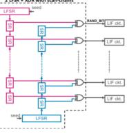
In order for network state to escape from the local minima, the stochastic computational annealing is adopted, using random walk by linear feedback shift register (LFSR).
