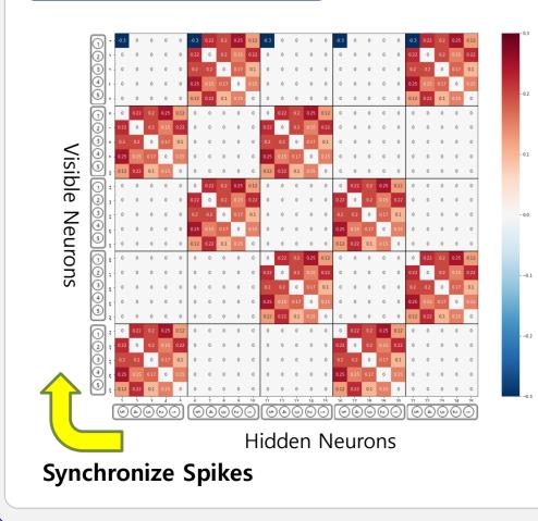
The conductance of PCM synapse that reflects the constraints (for TSP, the distance between cities) are set before neuron activation.
